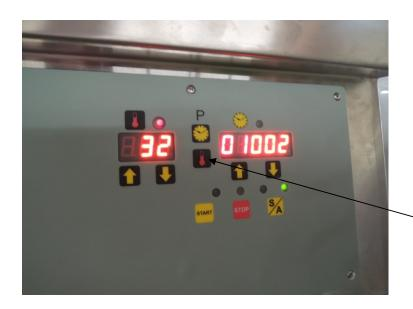
Pls press this Temp. setting key for the number dot moves forward to the next number when the right number is 9.
