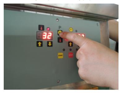
4. For example this display means the cycle time is 3,201,002. In fact you could set the cycle time very big numbers, so the machine would be not stopped when operation often.
