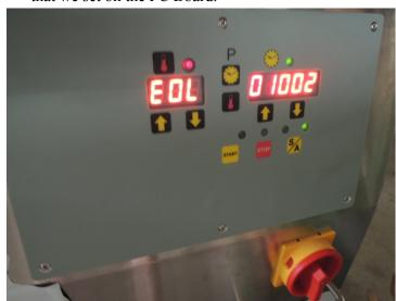
To Press the Increasing Key to clear the original setting time.
